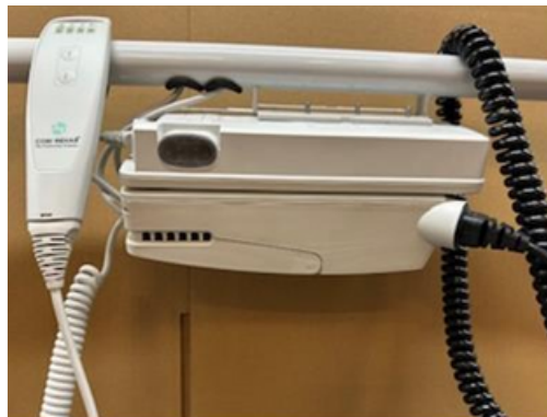
Battery is inside the control box.
