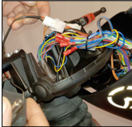
The plug from the potentiometer is now free.
