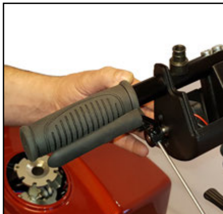
When the throttle handle is mounted, hold it in position "full speed" when you tighten the stop screw again.
