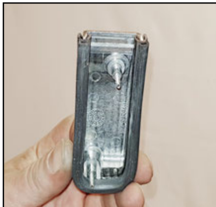
When the cover is to be mounted again, avoid pinching the cables.
