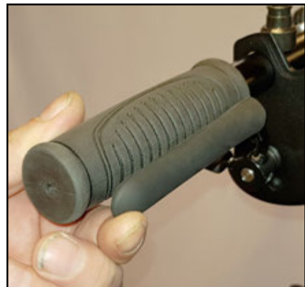
This means that the four-finger grip should touch the handle while tightening.
