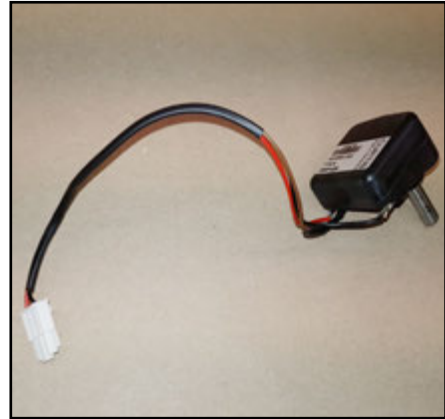
New potentiometer. Mount in reverse order.
