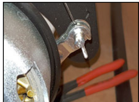
Shorten the brake cable, and fit a cable termination. Check that the brake function is working as it should.
