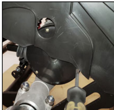
Remove the cover - three screws.
