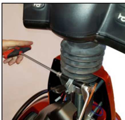
Dismantle the gas spring in the top area.
