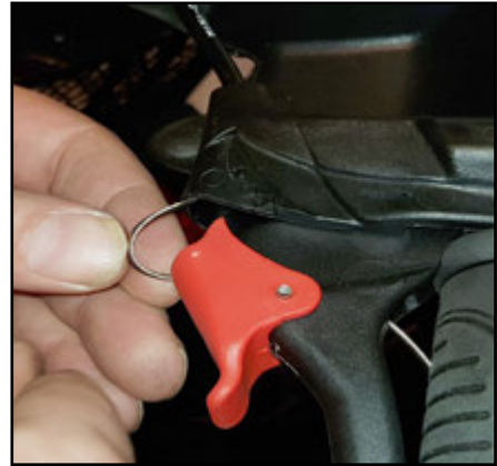
Push the cable all the way through the outer cable until it is visible by the rear wheel.
