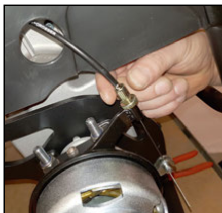
Fine tune the brake with the adjustment screw.
