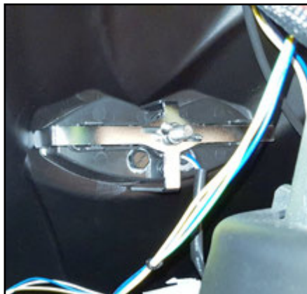
Mount the finger screw again.
