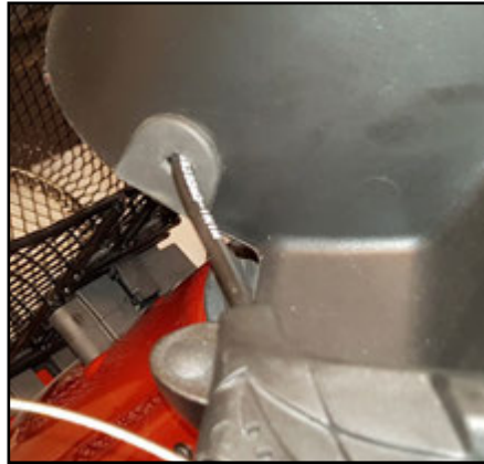
Mount the outer cable again.
