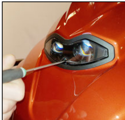
The headlight can be adjusted up/down by turning this screw.
