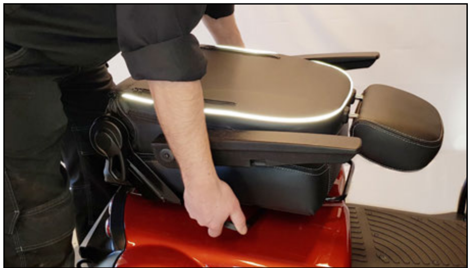
Lift the seat off the seat tube.
