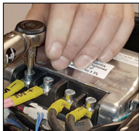
Mount the other plugs. Tighten with 5 Nm.
