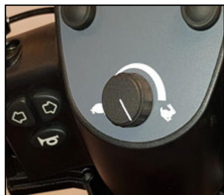
Turn the knob all the way to either the hare or the turtle before mounting the cover in correct position. Check that all functions are working.
