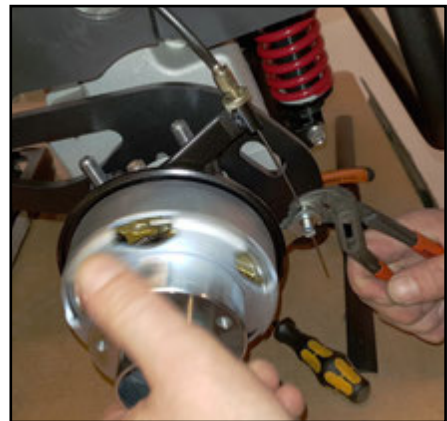
And through the small hole. Adjust the brake with the tool, while turning the hub. There must be no sound from the hub. When the hub just turn without sound, the cable can be tightened.
