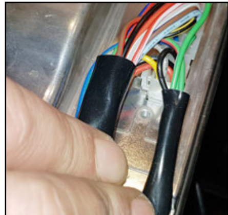
Make sure to move the cables, so the screw has access to the mounting hole.
