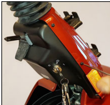
Remove the six screws that keep the cover in place.
