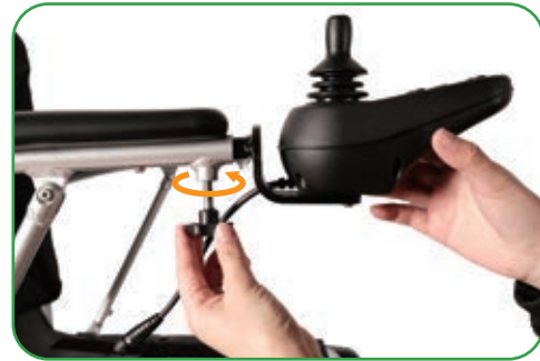
Photo 9. Secure joystick controller knob
