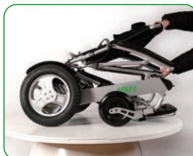
Photo 4. Expand the chair into a seated position
