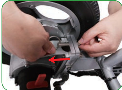
Photo 22. Remove the locking pin
