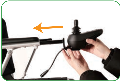
Photo 8. Slide joystick controller into armrest
