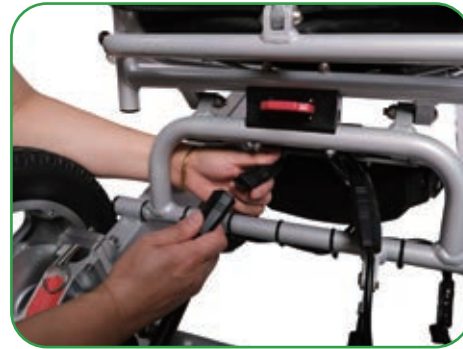
Photo 21. Release the rear wheels
