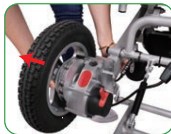
Photo 23. Slide out wheel assembly
