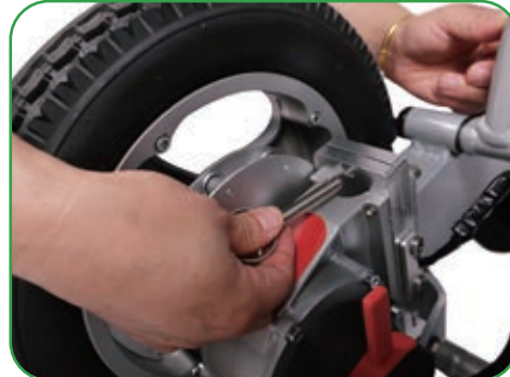
Photo 22. Remove the locking pin
