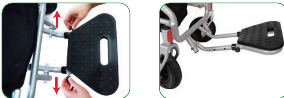
Photo 12. Adjust right foot rest length
