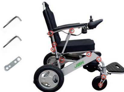
Photo 31. Check the screw loosening
