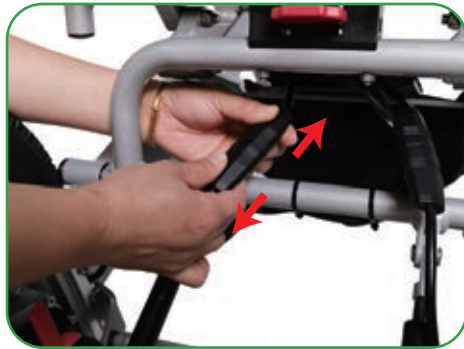
Photo 21. Release the rear wheels
