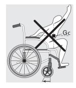
Do not extend your chest beyond the armrest (figure 4). In order to reach an object in front of you, you must lean and bend down; therefore, you must use the castors as a tool (pointing them forward) to maintain stability and balance. An accurate alignment of the wheels is essential for your safety (figure 5).
