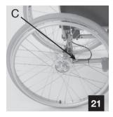
To adjust braking: turn the screw (C) counterclockwise to increase braking force and turn clockwise to reduce it.
