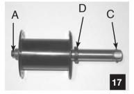
Always make sure that the spacer (D) is in place. Make sure that the axle and the locking balls are clean. (wipe out every month with a rag soaked with fine oil)
