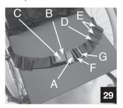
safety when using a reclining backrest, driving on slopes or crossing obstacles. These are removable: push down the button (A) and pull back. Reverse the procedure to reinstall. Make sure that the dog point (B) protrudes over the frame tube.
