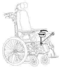
The depth is adjusted in a forward or backward position. Loosen handwheel (A) and turn.
