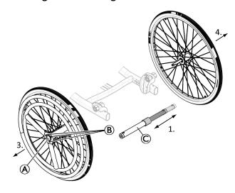
The removable and interchangeable rear wheels facilitate transport as well as change of the control side.
