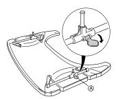
Open the safety lock for the depth adjustment (A).
