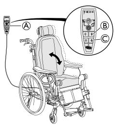
Tilt the seat unit (seat and backrest) by using the green buttons on the left side of the hand control (A).
