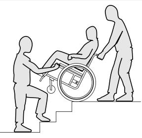
You can go up and down stairs by taking them one step at a time, as described above. The first assistant should stand behind the wheelchair holding the push handles. The second assistant should hold a solid part of the front frame to steady the wheelchair from the front.
