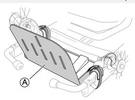
The ventilator tray (A) is a holder for various accessories such as ventilators, oxygen tanks, feeding units and so on. The ventilator tray can be adjusted 45 mm in depth and 120 mm in width in order to be adapted to various models.
