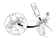
The armrests have an auto-lock to prevent involuntary movement or detachment. Press the button ® on the armrest to release before removing or adjusting the armrest.
