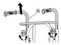
The push bar/push handles braced (A) must not be pulled up so that it protrudes more than 19 cm over the top edge of the attachment.
