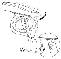
5. The hemiplegic armrest can be adjusted in angle. The resistance can be increased/decreased by adjusting the screw  $\widehat{\mathbb{A}}$ .
