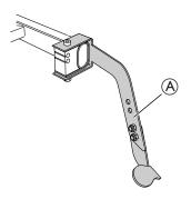
Use the kerb lever  $\ensuremath{\underline{A}}$  as a help when tilting the wheelchair backwards.
