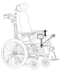
The height adjustment and removal is operated by the handwheel (A).
