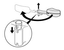
The "swing-away" trunk support can be turned sidewards in order to be out of the way when the user is moving in to or out of the wheelchair.
