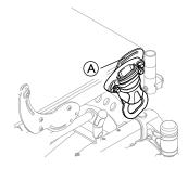
When using the belt for positioning of the knees, the front attachment slot 8 can be used.
