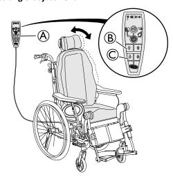
Adjust the angle of the backrest by using the yellow buttons on the left side of the hand control A.
