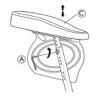
1. Loosen the screw (A).
