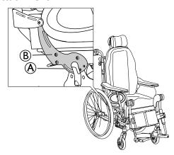
When using the belt for positioning of the thighs, the attachment slot a on the backrest attachment B can be used.
