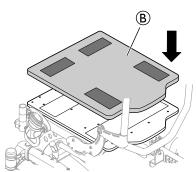
Place the height extension plate ® on the seat plate.
