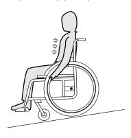
Lean back and carefully allow the handrims to run through your hands. You should be able to stop the wheelchair at any time by gripping the handrims.
