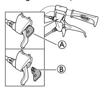
The locking device (A) allows you to set the tilting of the seat unit and/or the angling of the backrest to a fixed position.
