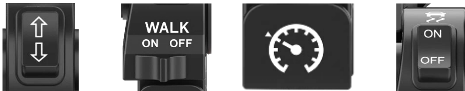
Figure 38. Switches and Indicators (L to R) Direction; Walk; Cruise; Traction.
