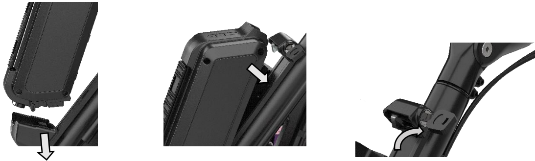
Figure 40. Inserting the Battery to the Battery Holder.
