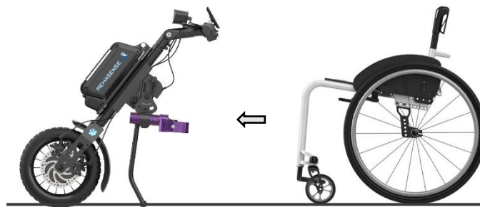
Figure 30. Roll the Chair to the Device
