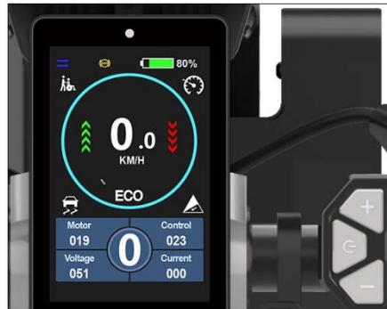
Figure 37. Power Device and Mode Selector Buttons
