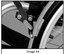
Wheel locks are applying correct pressure
