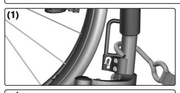
The wheelchair must be attached using a vehicle-anchored 4-point wheelchair restraint system in accordance with ISO 10542. These can be snap hooks, S-shaped hooks or snap fasteners. The wheelchair restraint system must be securely attached and used in accordance with the manufacturer's instructions for use. **(3A+B)**
