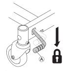
1. Lock the brakes: Push down the pedal (A).
