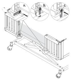
Pull out the pin, rotate anti-clockwise by 90 degrees and release it to position the tab in the vertical slot.
