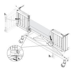
Press the levers on the underside of the side rail and open the folded doors.
