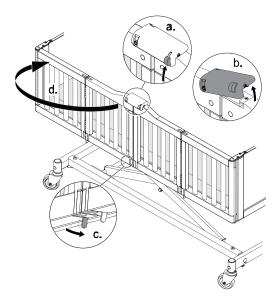
Push up the knob and lift the latch. While holding up the latch press the corresponding lever on the underside and fold the door.
