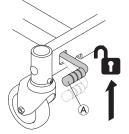
2. Unlock the brakes: Pull up the pedal (A).
