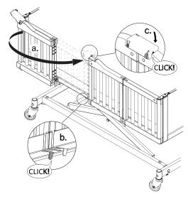
Unfold the door with the latch on the top bar and ensure the locking mechanism on the underside and at the top bar engage with an audible click.
