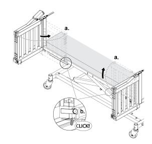
Close the folded doors and ensure the locking mechanisms on the underside engage with an audible click.
