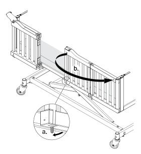
On the other door, press the lever on the underside and fold the door.
