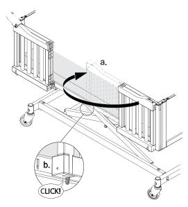
Unfold the door without the latch on the top bar and ensure the locking mechanism on the underside engages with an audible click.
