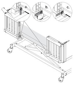
Pull out the pin, rotate clockwise by 90 degrees and release it to position the tab in the horizontal slot.
