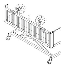
3. Slightly lower the side rail and release the two latches.
