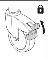
**Locking the brake** - Step on the outer pedal ® **Unlocking the brake** - Push up the release button ®
