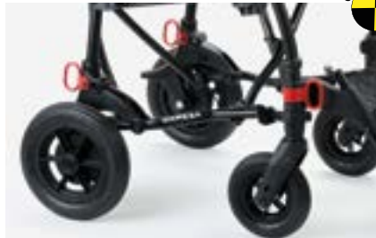
891 Set of 4 tie down hooks for the forward-facing transport of the pushchair in a motor vehicle (private/ cars, buses..). See User and Maintenance Manual provided with the aid.
