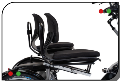
Seat console w/ inclination (2) – fits both standard and junior seats - 5011215
