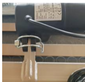
Quick-release pin to fix the actuator
