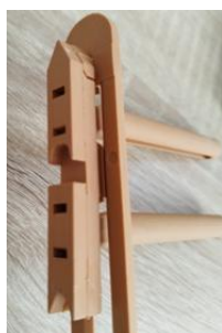
Side rail top locking button/ fixator
