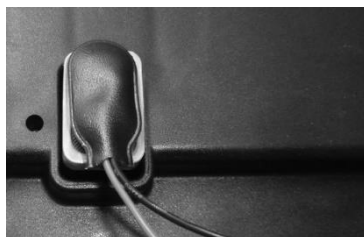
9V block battery for emergency lowering
